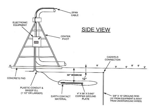
Ground rods are to have a minimum diameter of 5/8" and a minimum length of 10 feet. These are to be driven into the ground in a vertical position or an oblique angle not to exceed 45 degrees at a location 10 feet from the electronic equipment and the wires and cables connected to the center pivot. The ground rod is to be stamped with the UL logo. The ground rod should be connected to the ground lug located inside the control panel enclosure using a 6 AWG solid bare copper wire.
