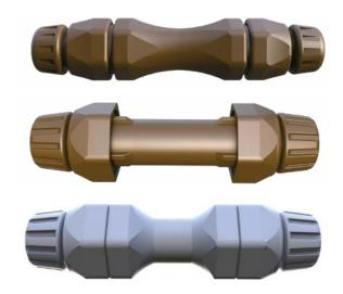
The Melni Connector can be installed in less than one minute! Just insert the stripped cable, twist the end caps to tighten the patented spiral insert and then tighten the waterproof caps. That's it!
